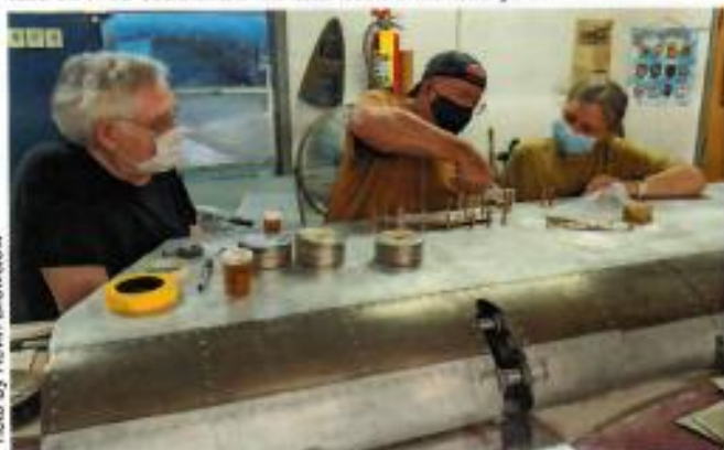
Dennis Smirt and Deb Lamere watch as Joe Wulfskuhle patches the F-86H flap
